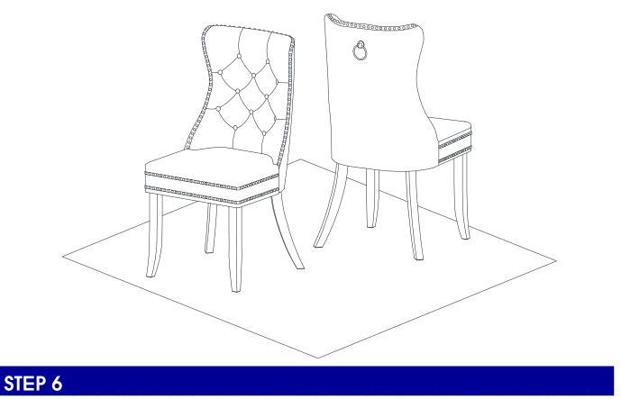
Attach the bottom cover (removed on step 1) back on the seat frame and finish the assembly.
